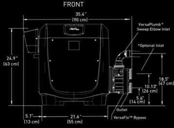
NOTE: Dimensions are identical on all heater models
